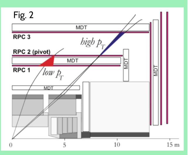
Each RPC detector consists of two gas gaps (2mm width), read-out by two orthogonal planes of strips, in  $\eta$  and  $\Phi$  views, with a
