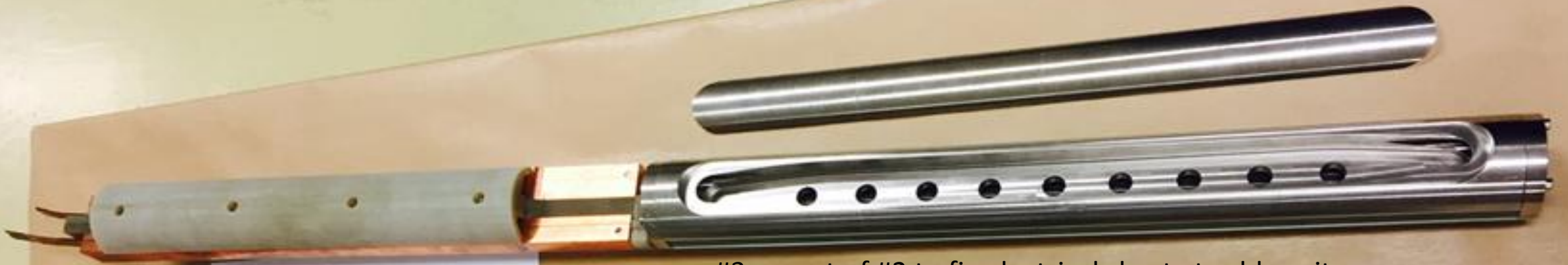
#3 repeat of #2 to fix electrical short at cable exit
