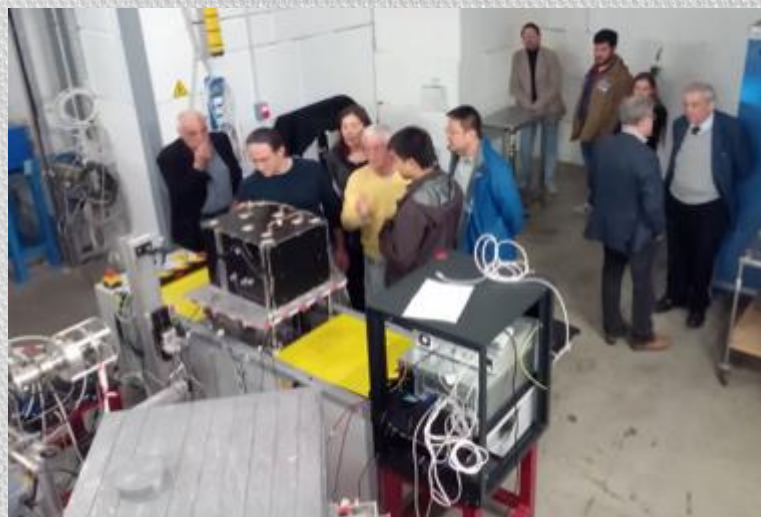
Test of High Energy Particle Detector (HEPD), for low energy electrons (3-100 MeV), protons (30-200 MeV) and light nuclei with high angular and energy resolution: LYSO calorimeter + Si micro-strip detectors
