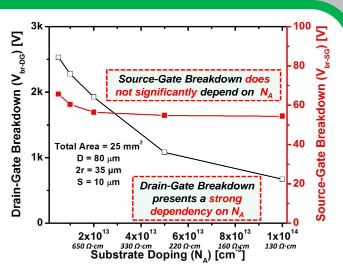
**Edge termination techniques** (floating guard Rings, deep N-type diffusions, P-Spray....) are considered to recover the breakdown values
