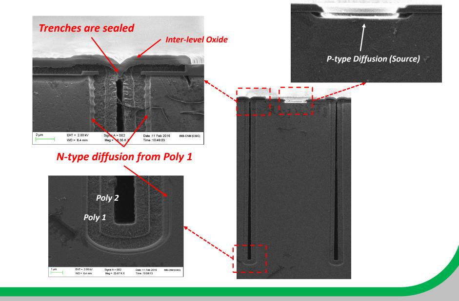
Narrow Channel Devices  $(2r = 23 \mu m; s = 10 \mu m)$
