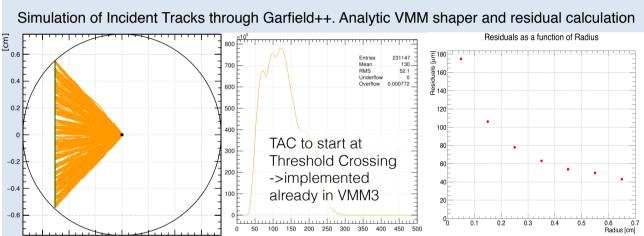
Resolution is basically noise limited and shorter integration time  $\sigma_t = \frac{ENC}{Q} au_{peak}$ would result in higher resolution. The charge collected in 15 ns is ~80% of that collected in 25 ns. VMMx will include a 15 ns peaking time in addition to the four already existing.
