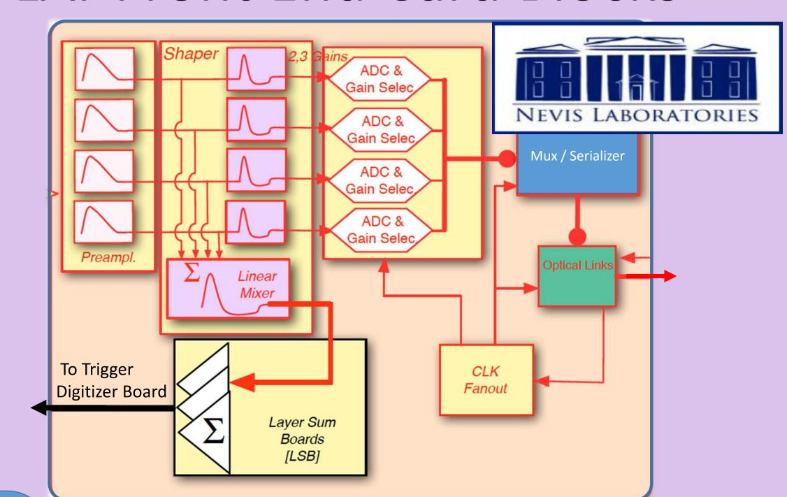
Preamp Requirements: Input termination selectable  $25\Omega$  or  $50\Omega$
