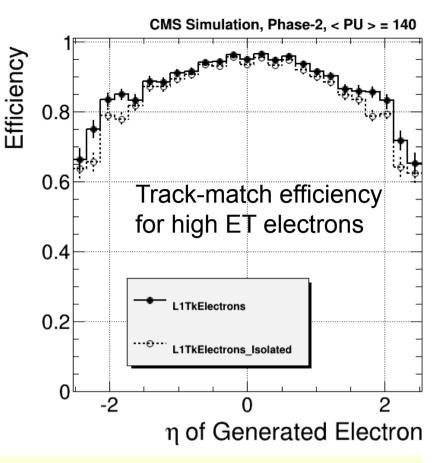
For an efficiency of > 90% in the central region: track-matching reduces the rate of a single-electron trigger by O(5) at 20 GeV
