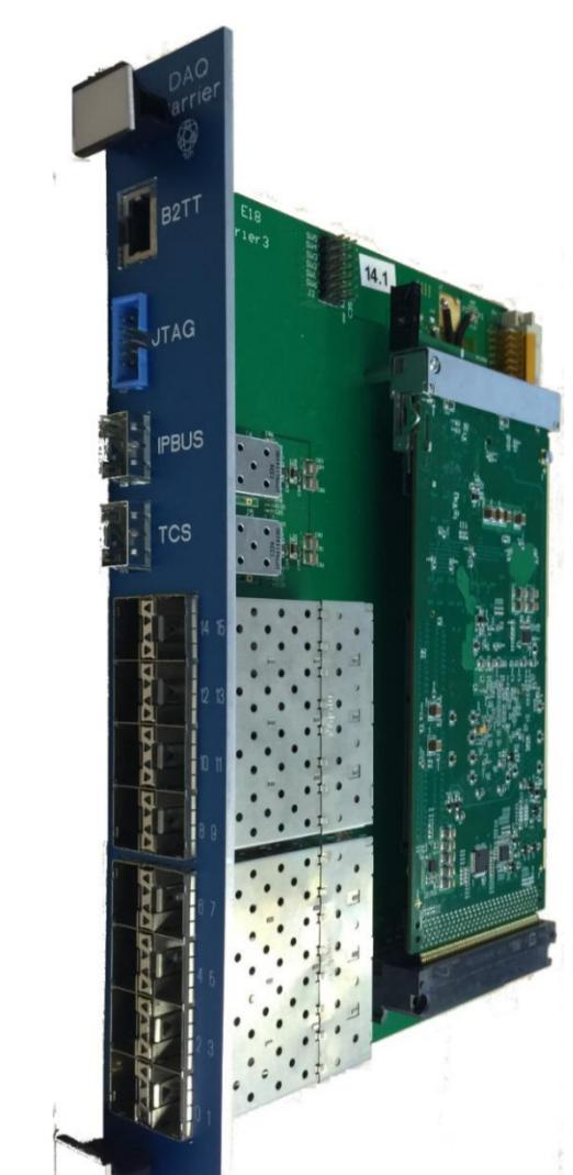
DHC on VME carrier Card as used for DHCmx and DHCsw
