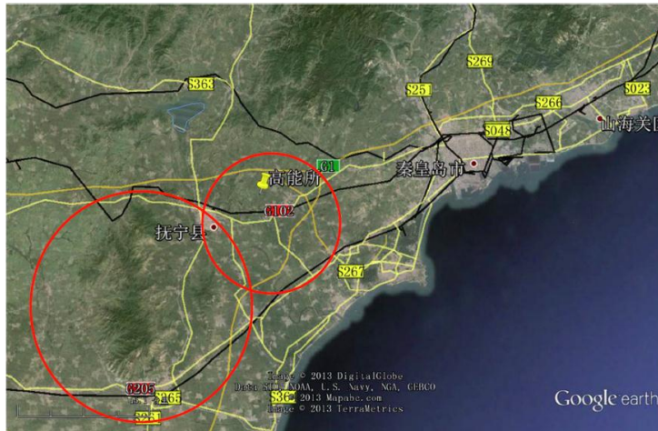
Figure 3.3: Illustration of the CEPC-SPPC ring sited in Qinhuangdao. The small circle is 50 km, and the big one 100 km. Which one will be chosen depends on the funding scenario.
