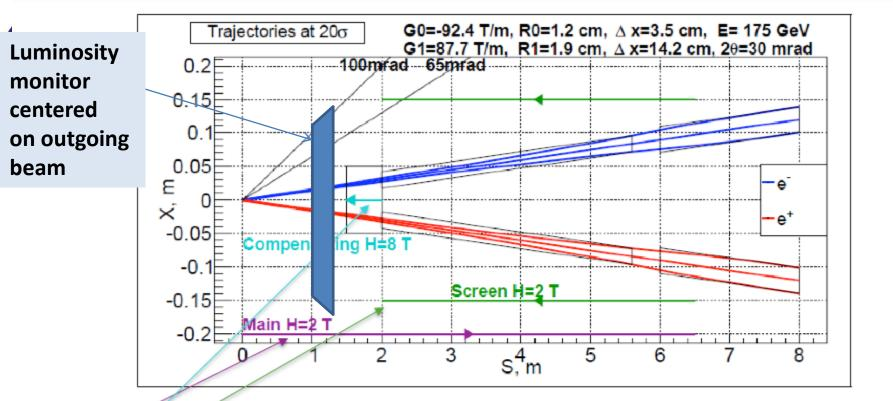
Beams are crossing detector B-field at an angle of 0.015 mrad. Need compensation.
