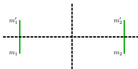
Figure: Graphical representation of the blocking of the A tensors. The vertical tensors are the A^{(s)} and the dashed lines are the links of the original lattice.
