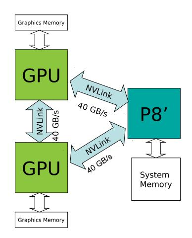
GPUs Bottlenecked by PCIe Bandwidth From CPU-System Memory NVLink Enables Fast Unified Memory Access between CPU & GPU Memories
