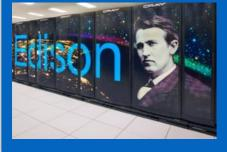
5576 Nodes 134k CPUs Intel Xeon Ivy Bridge 24 cores / node 64 GB RAM / node 7.6 PB SCRATCH /project: 9.1 PB quota-based GPFS, for long term storage (not optimized for I/O)
