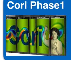
1630 Nodes 52k CPUs Intel Xeon Haswell 32 cores / node 128 GB RAM / node 28 PB SCRATCH 750 TB Burst Buffer
