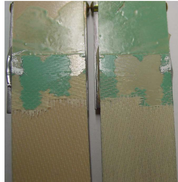
component failure, interlaminar inside the composite
