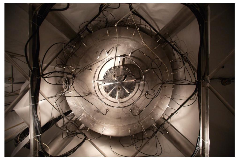
• DarkSide searches for WIMPs using a liquid argon detector immerse in a liquid scintillator veto and in a water tank
