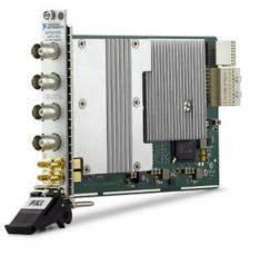
Done using LabVIEW and new custom API made for the NI PXIe-5162 digitizer
