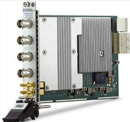
PXIe-5162 4ch, 1.5GHz, 10-bit Digitizer
