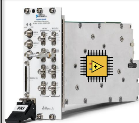
PXIe-5646R 6GHz Vector Signal Transceiver
