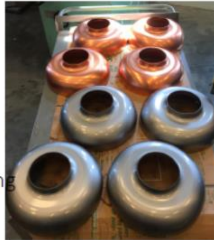
Deep-drawn 802 MHz Nb and Cu half-cells (Status April '17)
