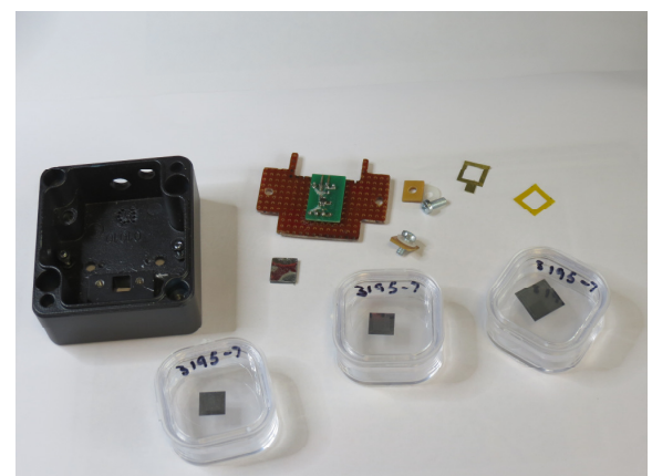
Avalanche test sensors fabricated by Micron Semiconductor under assembly at Diamond Light Source for the first tests with radioactive sources.
