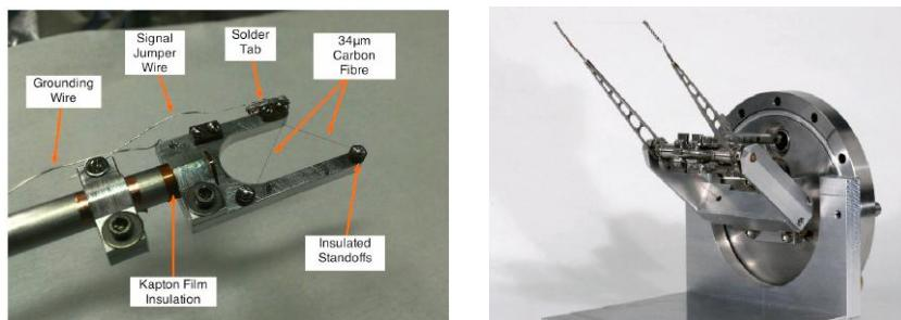
Fig.1 A carbon (left<sup>1</sup>) and metal (right<sup>2</sup>) based wire scanner at the present employed in the FEL, collimators and synchrotrons beam lines
