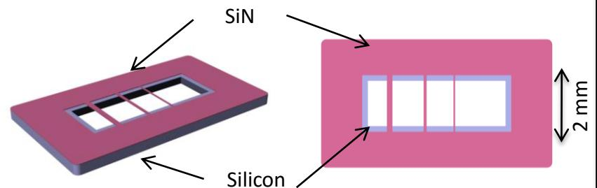
Fig.2 Scheme of the proposed device
