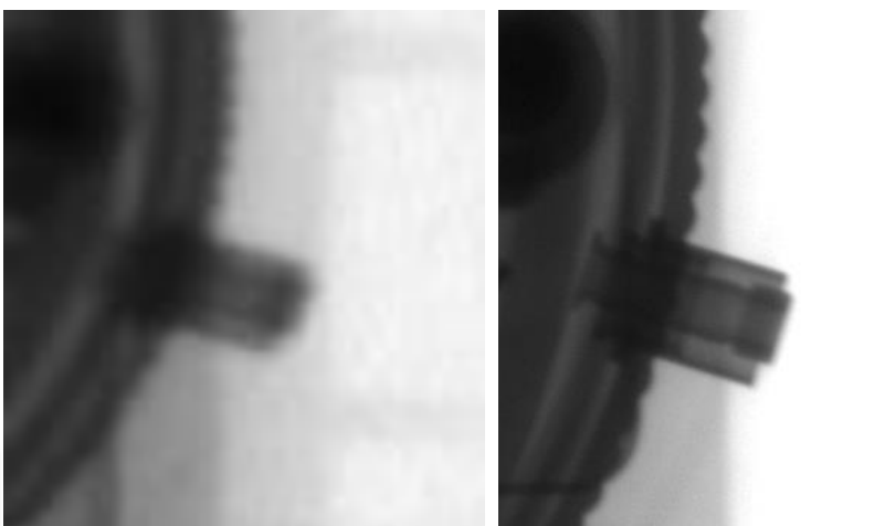
Fig.7. Part of radiogram acquired by standard 200 \mu m resolution linear detector (left) and high resolution fluoroscopic detector (right)
