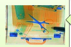
This will provide colored X-ray pictures. Combined with X-ray absorption spectroscopy, it will allow for identifying material signatures in pictures (e.g. copper, iron).
