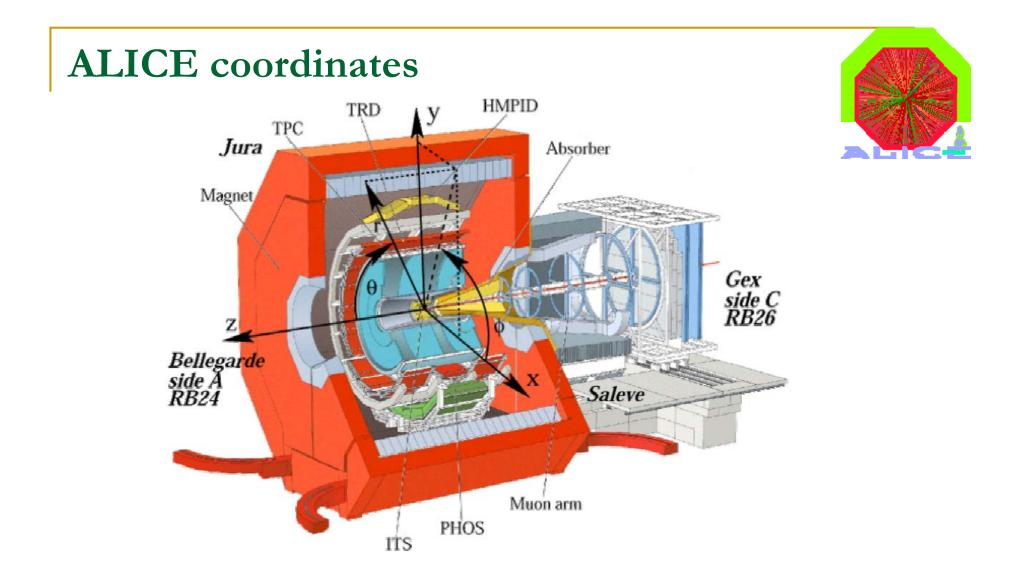
Fig1. Definition of the ALICE coordinate system axis, angles and detector sides.
