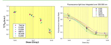
The plastics transmit and yield less light with an increase in dose. Not much difference can be seen between samples<sup>7</sup>.
