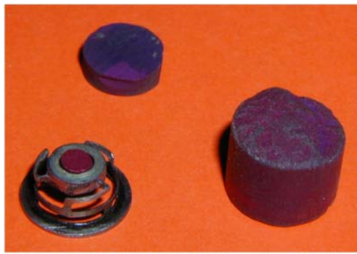
cathodes damaged by sputtering
