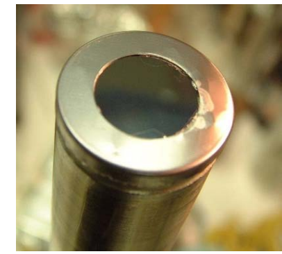
Stalk for supporting 1 Photocathode
