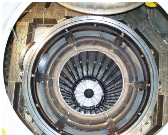
Fig. 16: The CERN's large furnace dedicated to vacuum firing of austenitic stainless steels. Useful height and diameter: 6 m and 1 m, respectively. Maximum charge weight: 1000 Kg. Ultimate pressure: about 10^{-7} mbar; pressure at the end of the 950°Cx2h treatments: 10^{-5} mbar.
