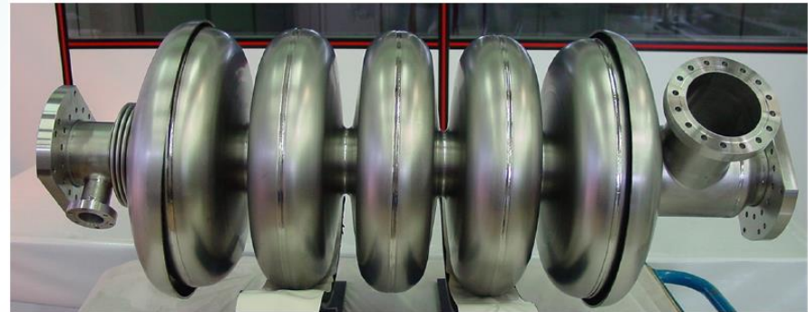
\beta = 0.65, 704 \text{ MHz} elliptical cavity
