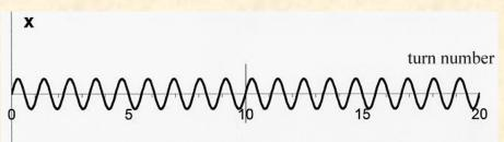
10 turns in the cyclotron for 9 horizontal oscillations  $v_r\omega_0 < \omega_0$  (9/10 = 0.9 =  $v_r$ )
