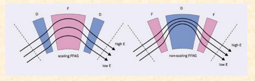
The orbit shape is invariant in scaling FFAG cells, but varies with energy (E) in non-scaling ones (F = focusing, D = defocusing).
