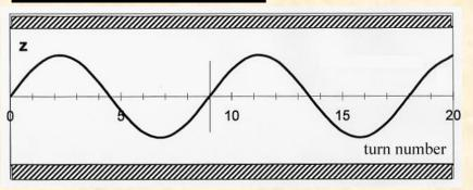
1 vertical oscillation for 9 turns in the cyclotron  $v_z \omega_0 < \omega_0$
