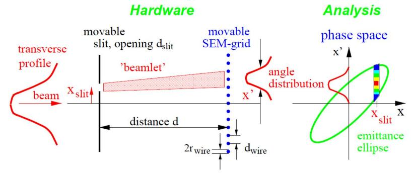
*Slit*: position P(x) with typical width: 0.1 to 0.5 mm
