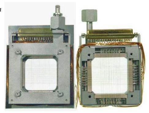
Each wire is equipped with one I/U converter different ranges settings by  $R_i$
