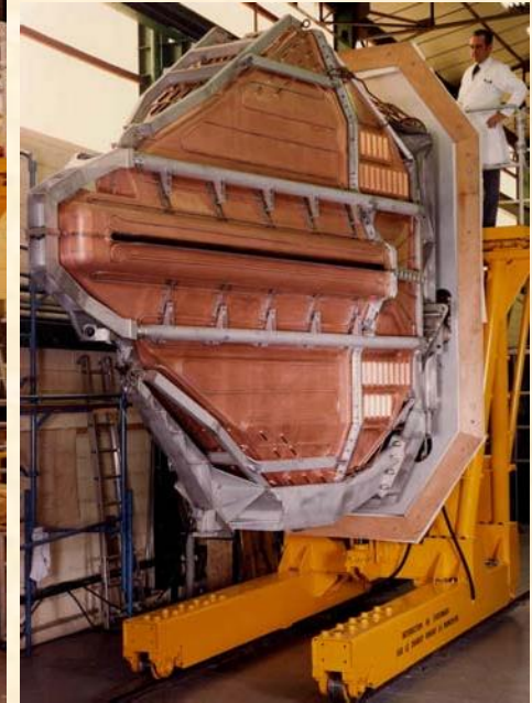
Outer shell of resonator, with support frame and beam slit
