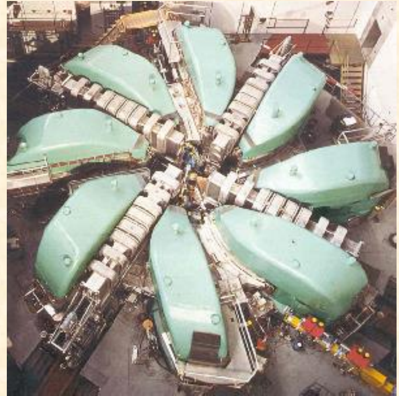
Typical 'Separated Sector Cyclotron' (SSC), median plane view (left), and photo (right). Shown is the PSI 590 MeV (p) ring cyclotron, with 8 sector magnets and 4 accelerating cavities
