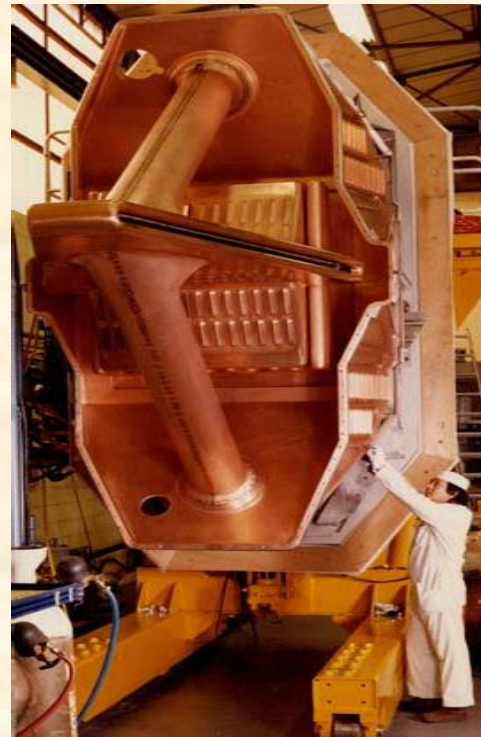
Copper skinned inner conductors with 'Dee' (inner electrode)
