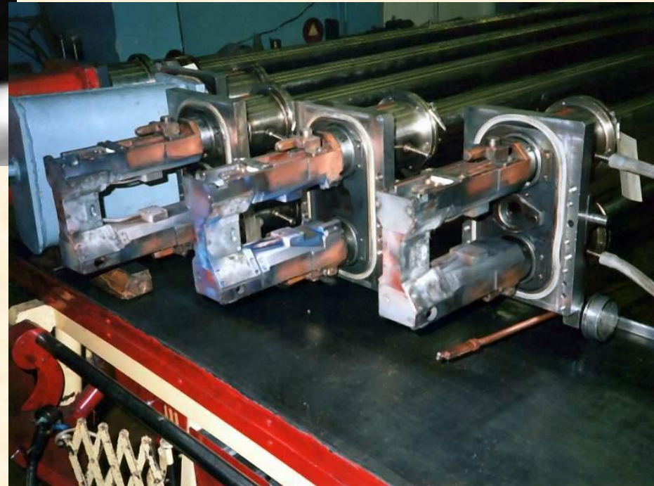
FLNR, PIG test-bed, 1992. The head of MC400 cyclotron vertical ion source
