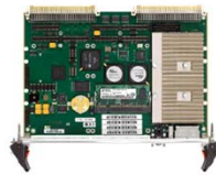
VME Card: Eurocard size VMEbus interface
