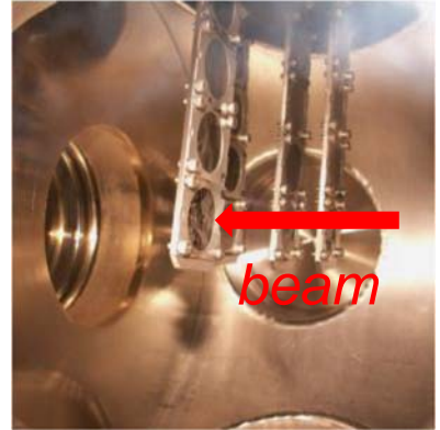
Carbon foil at CERN LINAC3
