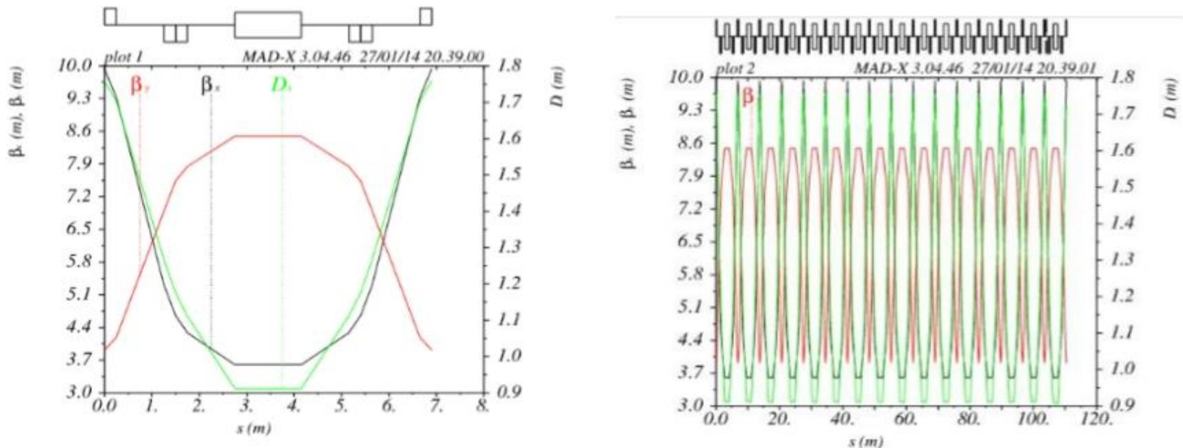
It uses only bending magnets (no long straight sections)
