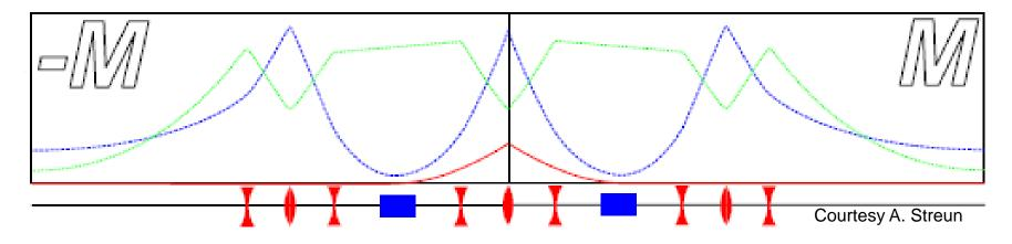
This is the basic structure of a DBA lattice used in many light sources
