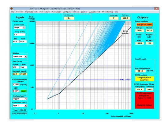
And with 10 kW travelling wave power=10 watt RF generator power for Q=100 you are really in the red area...
