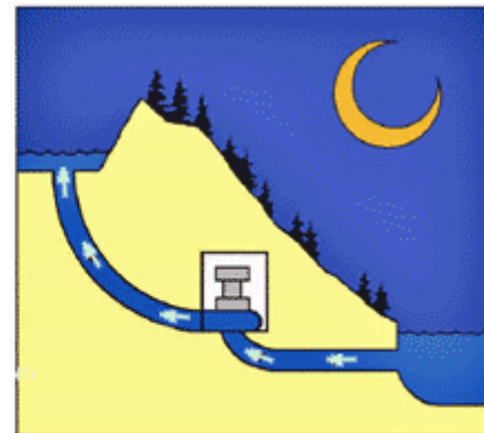
Nighttime: Water pumped uphill to reservoir for tomorrow's use
