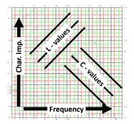
Find the intersecting point of frequency and Characteristic impedance. Then look for diagonal lines passing close to this point. Read the L and C values from these lines and enter this initial guess into the applet. Now you can find a more accurate solution by fine tuning the values.
