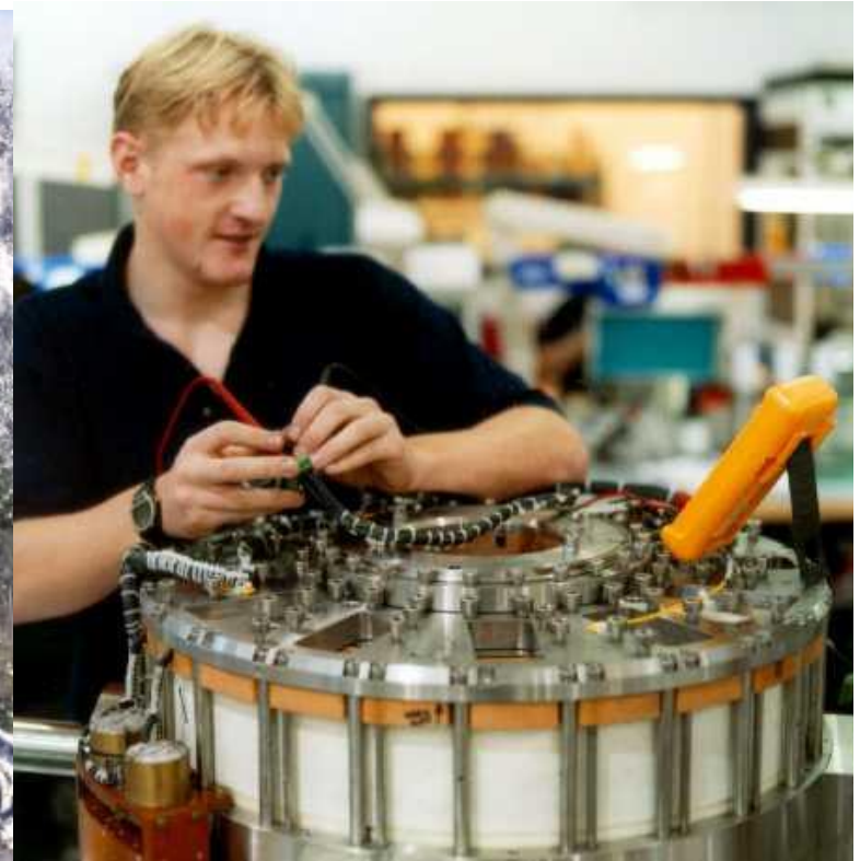
Superconducting solenoid for research
