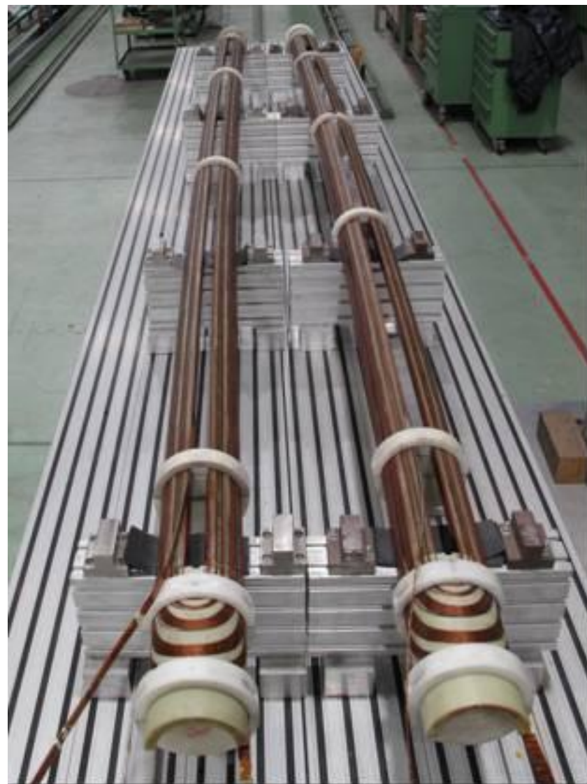
Discorap curved dipole INFN Frascati / Ansaldo
