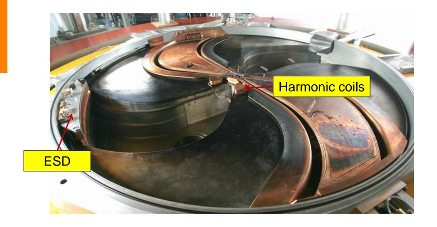
Spiral sectors => better vertical focusing Elliptical gap => high B-field and easier extraction
