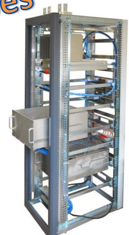
4-quadrant for correctors : \pm 200A/\pm 10V \pm 2kA/\pm 10V
