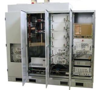
4-quadrant for correctors : \pm 200A/\pm 10V \pm 2kA/\pm 10V
