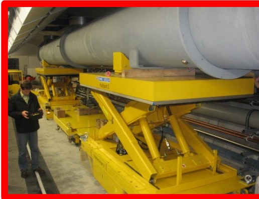
DESY XFEL installation Capacity: 6.t per lifting platform Lifting height: 2.4m
