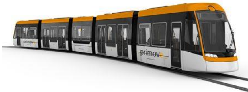
Supercapacitor recharge at periodic stops
