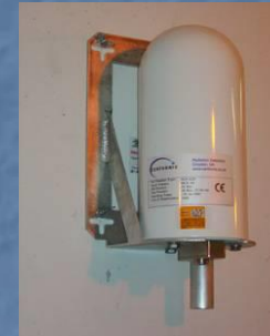
High pressure ionization chamber
