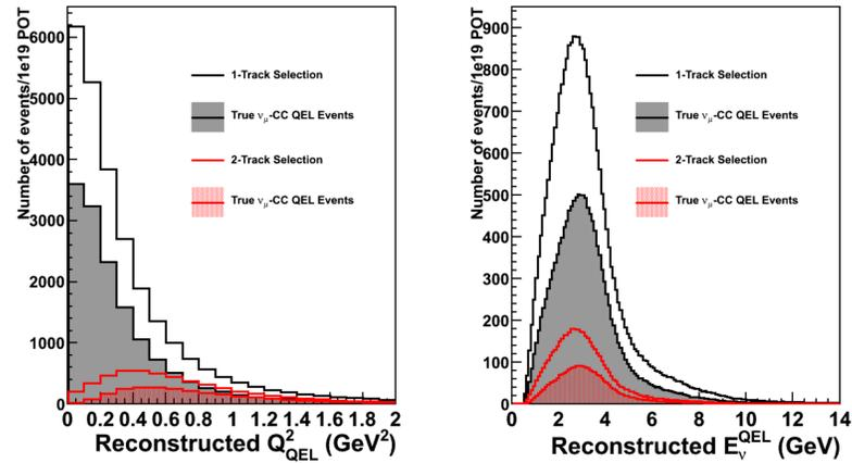
There are two channels for the detection of QE interactions. In the 1-track channel (on the left), which is used in the preliminary MINOS QE results, the recoil proton is below detector threshold. In the 2-track channel (on the right) the recoil proton is above detector threshold and leaves a reconstructable track.
