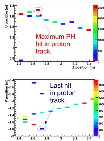
Protons lose most of their energy at the end of their track. Thus we require that the highest pulse height hit in the candidate proton track is within 1 plane of the last hit in the candidate proton track.
