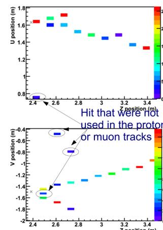
We expect that QE events should have very little vertex activity out side of the reconstructed muon and proton tracks. Thus we require that the number of hits that were not used in either the muon track or the proton track be less than 6.
