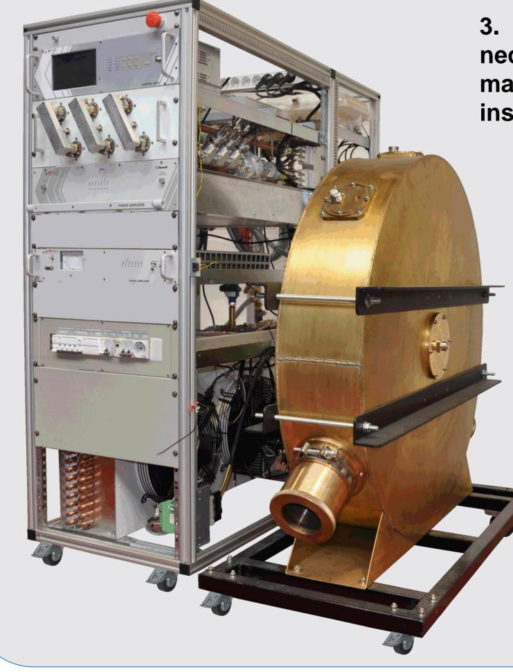
3. Test bench, designed by BTESA, necessary to replace the functions of the main SSPA control, circulator, loads and
