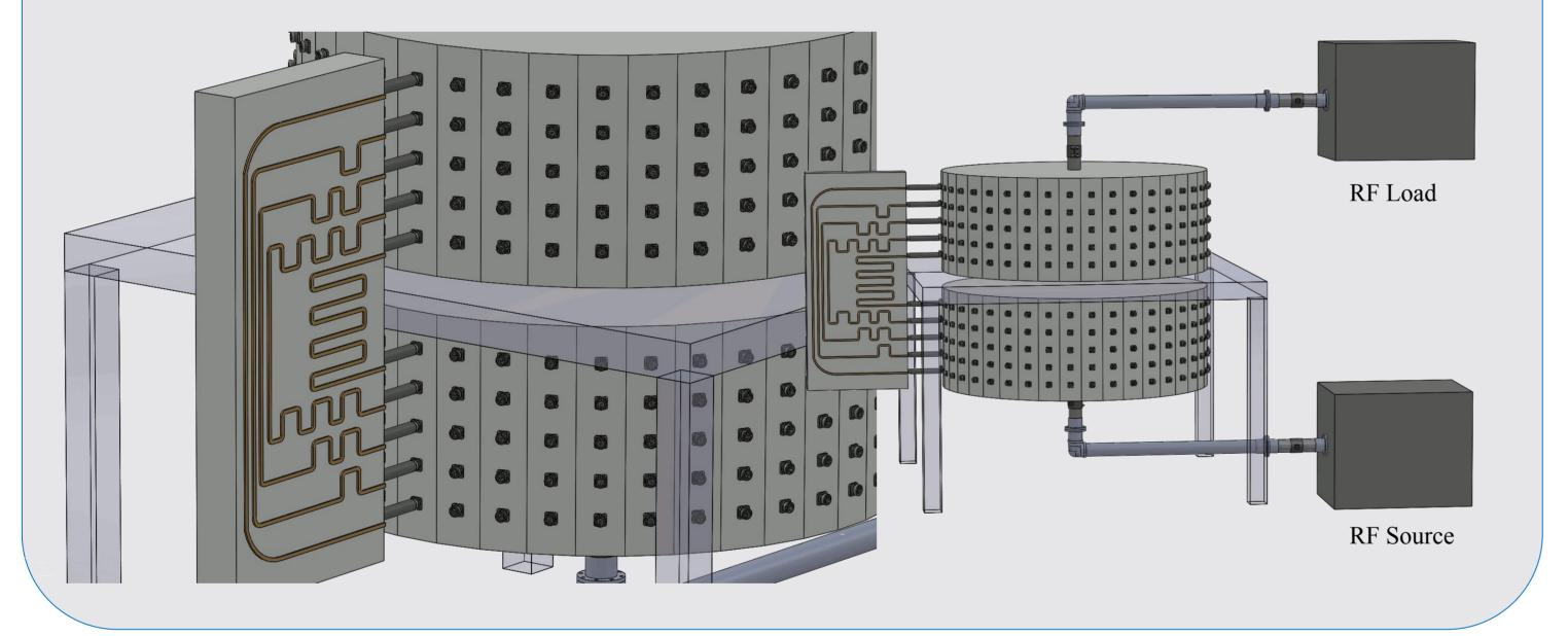
Some auxiliary RF tasks such as conditioning of cavities or couplers need temporary RF power systems.
