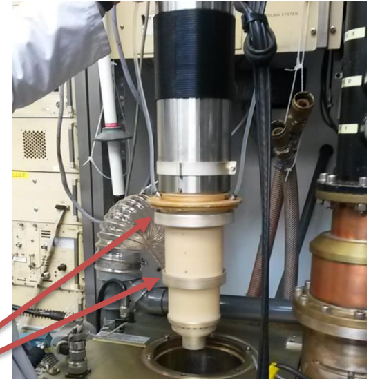
TH795 with upper adaptation ring installed
