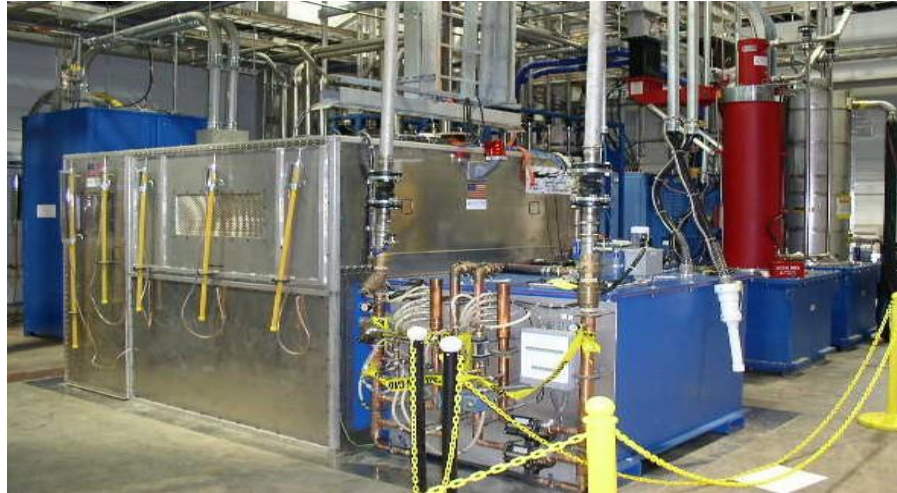
High-Voltage Converter Modulator (Alternate Topology)
