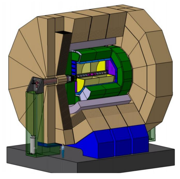
The ILD detector systems have many layers surrounding the point where the beams collide
