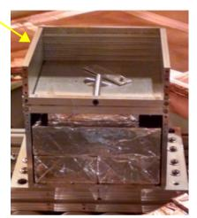
γ source and Be wafer in fixed position:
