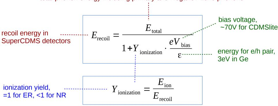
Accurate  $E_{\text{recoil}}$  measurement requires knowledge of  $Y_{\text{ionization}}$ :
