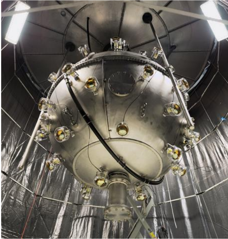
Completed Detector: Steel Shell, calibration tubes, muon veto in Shield Tank (fall 2015)
