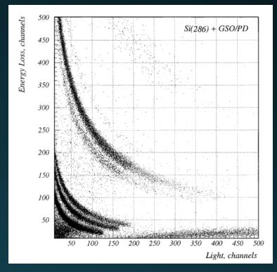
Need detailed calibration of the response of crystals as a function of nucleus (A,Z) and energy.
